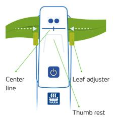
Press the measuring head together by using the thumb rest. Hold until the LED blinks. You will also be notified on your smartphone.
