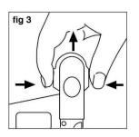
4) Slide the test disc under the measuring head. Squeeze the measuring head until a beep sounds and a reading appears in the display. If a series of beeps sounds and "---" appears in the display, the measurement was not performed correctly. In this case, repeat step 4 (Fig.4).
